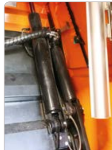
Interior carriage plate cylinders
