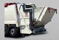
• Folded down: Low feeding height for hand-loading of waste
